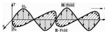
Figure 6. The planar electromagnetic wave in the far zone.
